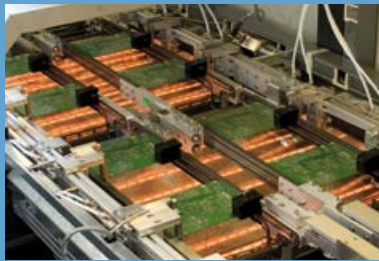
Dual track conveyor
